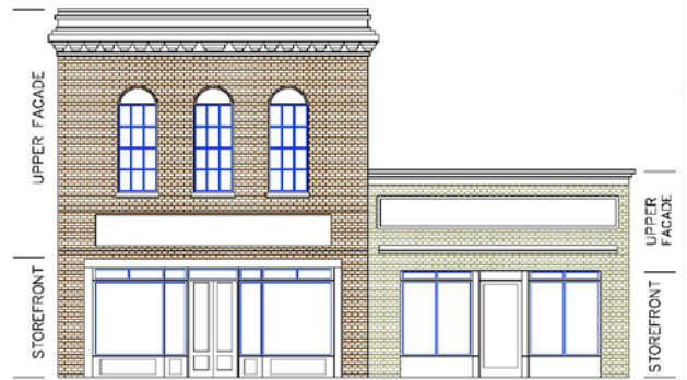
Elements of the commercial façade.
