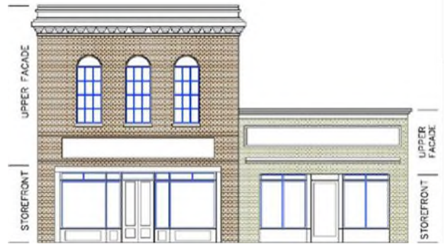
Elements of the commercial façade.
